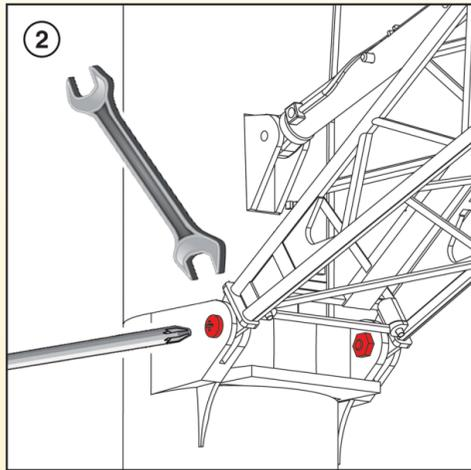
Position the boom at the desired position and if necessary retighten the screw at the boom fulcrum point.
