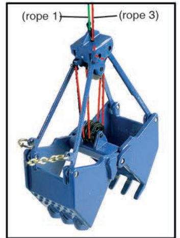
05. fix and rope-up respectively the grabber ropes (1) and (3)
